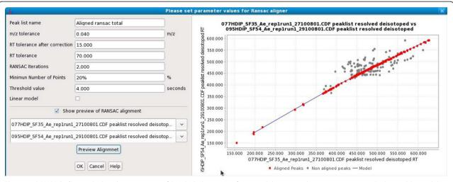
**Figure 5 RANSAC aligner**. Dialog shows preview of RANSAC alignment of two peak lists using the given parameters. Each possible candidate alignment (peak pair) within a defined m/z and retention time tolerance is shown as a dot. A model is fitted to the data (blue line) and red dots indicate those fitting to the model and therefore selected for the final alignment.
