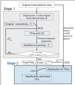
**Figure 1** A schematic overview of the method. The TFA perturbations are estimated in an iterative fashion that trims unimportant edges from the regulatory (connectivity) network. If the data set is not NCA-compliant, additional data are generated *in silico* before estimating the TFA perturbations. Then, the significance of the TFA perturbations is assessed using the z-test and null distributions created by random sampling of expression data across the whole genome.
