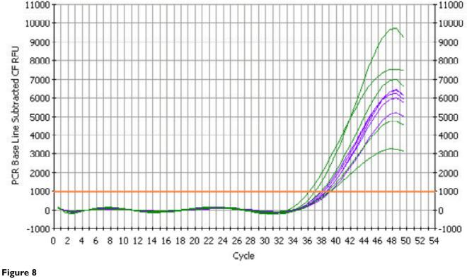
**Optical factors affect the plateau scattering**. SYBR Green real time PCR in frosted plates (green) and white plates (blue). Frosted plates cause increased plateau scattering because of inconsistent reflection and refraction (Reproduced from [18], with ABgene<sup>®</sup> permission).
