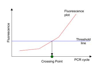
Figure 2 Direct calculation of crossing points.
