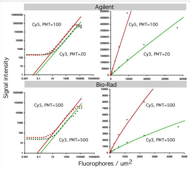
**Figure 2 Comparison of PMT responses for different channels and gains for Agilent (top row) and Bio-Rad (bottom row) scanners.** Left column shows data in log-log coordinates, right column - in original non-transformed coordinates.
