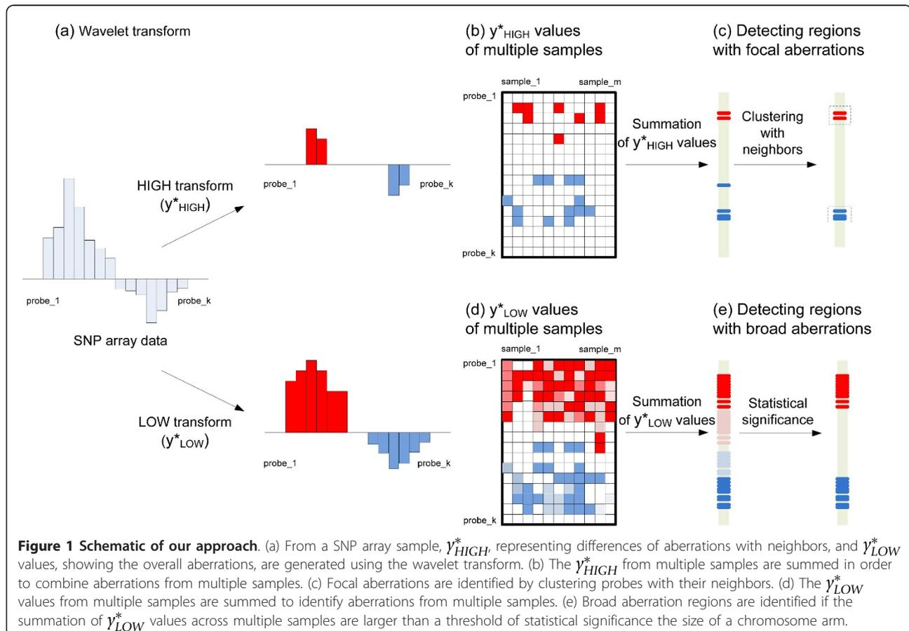
and it repeats this process recursively, pairing up the averages to provide the next level—finally resulting in  $2^L$  averages (stored in the scaling coefficients  $s$ ) and  $2^J - 2^L$  differences (that are stored in the wavelet coefficients  $w$ ). For more details about wavelets, refer to [23], [24], and [25].
