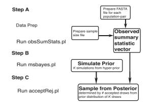
Figure 2 Flowchart describing operation of msBayes.
