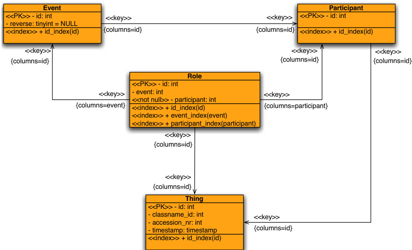
Figure 2 Simplified DDL Diagram of BNDB. The simplified structure of the database schema.
