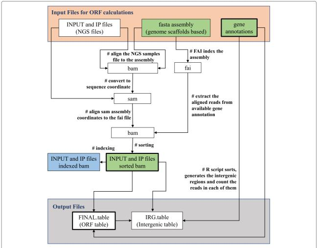
**Fig. 1** Core RACS pipeline overview. This flowchart represents the logic steps implemented in the core pipeline. Boxes represent files and file types as indicated in the text. Files with thick boxes represent the Input Files for Intergenic calculations. Files in green are to be uploaded to IGV. File in blue is needed for IGV but it does not have to be uploaded to IGV. This file has to be kept in the same folder directory than the sorted bam
