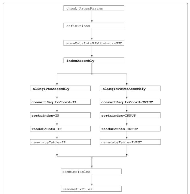
**Fig. 2** Schematic diagram of the tasks implemented for the RACS core pipeline. Included are details of the processing stages in relation to the scaffold based genome and the breakdown of each these steps. Bold names, indicate bioinformatic specific modules while normal fonts represent generic ones. The bifurcation represents tasks that can be executed in parallel, as there is no data dependency among them
