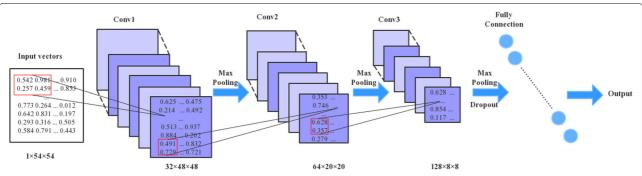
Fig. 2 The architecture of our convolutional neural networks. This topology is similar to LeNet-5 networks which contains three convolutional layers, two pooling layers and one fully connected layer
