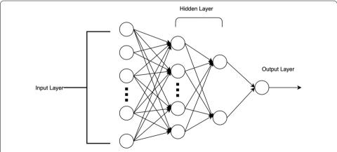
**Fig. 2** The illustration of the neural network structure. The structure of a deep neural network, which contains two hidden layers and the output layer is a sigmoid function
