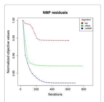
**Figure 5 Plot of the residual approximation error**. Each curve reports the trajectory of the approximation residuals, computed with the algorithm's loss function. Each track is normalized separately over its maximum value, and stops at the number of iterations required to achieve the convergence criterion.
