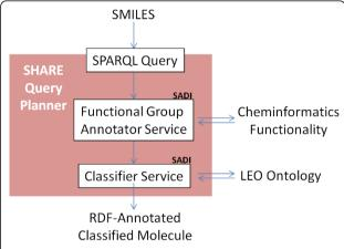
**Figure 1 Summary of the proposed core lipid classification framework.** A SMILES description of molecular graph for a given chemical entity is submitted to the SHARE client, which automatically identifies and orchestrates the execution of the annotation and classification SADI services. The output is an RDF graph that contains classification and functional group annotation of the input chemical entity.
