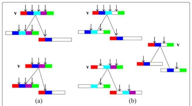
**Figure 10 (a) Non-gapped segments (b) Gapped segments** t-coalescent vertex v: Five cases are shown where the total number of junctions does not increase with coalescence. The white segments represent the gaps whereas the colored segments refer to the non-mixing segments. (a) Two cases with non-gapped segments. (b) Three cases with gapped segments.
