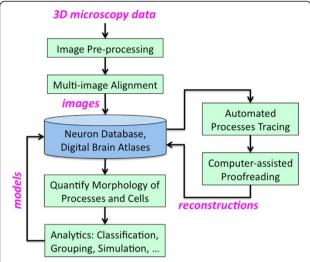
**Figure 1 Major steps in building digital neuronal databases and brain atlases.** After necessary image processing, the 3D morphology of a neuronal pattern is reconstructed from microscopy data. Multiple neuronal patterns need to be organized based on brain regions and neuronal types. For brain atlases, these reconstructions are mapped into a common 3D spatial coordinate system. This may involve an iterative analysis process.
