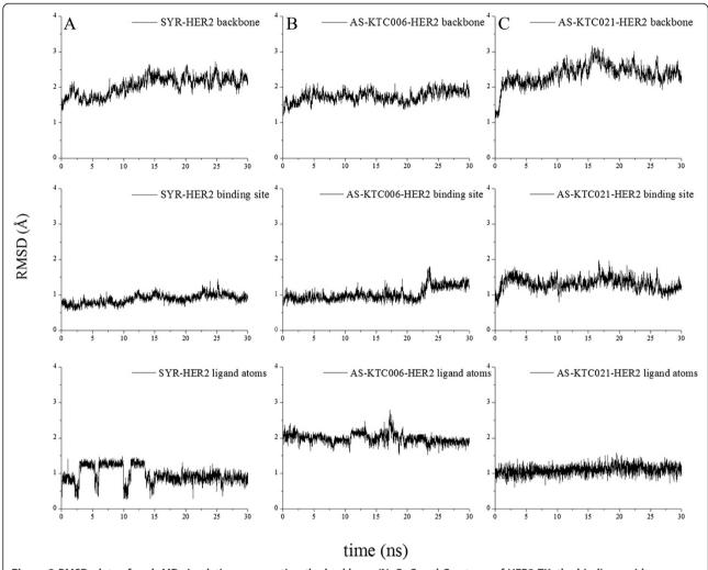
Figure 3 RMSD plots of each MD simulations, presenting the backbone (N, O, C and C $\alpha$  atoms of HER2-TK, the binding residues atoms of HER2-TK and ligand atoms in upper, middle and lower rows, respectively, in the panel of A) SYR B) AS-KTC006 and C) AS-KTC021.
