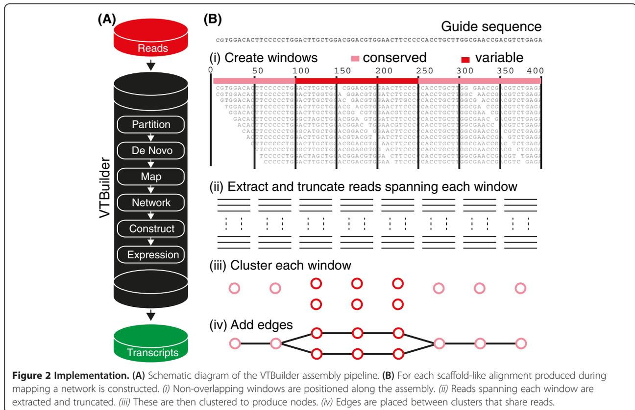
**Figure 2 Implementation.** (A) Schematic diagram of the VTBuilder assembly pipeline. (B) For each scaffold-like alignment produced during mapping a network is constructed. (i) Non-overlapping windows are positioned along the assembly. (ii) Reads spanning each window are extracted and truncated. (iii) These are then clustered to produce nodes. (iv) Edges are placed between clusters that share reads.
