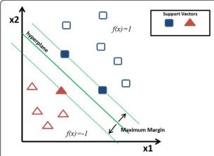
Figure 1 Two dimensional representation of support vector machine, using maximum margin with support vectors to classify data. Local model is generated for each transcriptional factor to classify list of genes.
