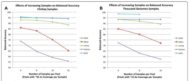
**Fig. 1** Effects of Pool Size on Program Balanced Accuracies. "Balanced accuracy" is defined as the mean of the sensitivity and 1 minus the false positive rate. No data point is reported for GATK with 16 or 32 samples because runs did not complete within a reasonable timeframe. Values are plotted for (a) ClinSeq and (b) Thousand Genomes pools containing read depth 50 % of a typical whole exome, which was 35.1x, on average, for ClinSeq samples and 21.0x, on average, for Thousand Genomes samples
