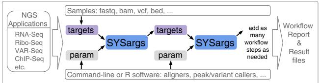
**Fig. 1** Workflow steps with input/output file operations are controlled by *SYSargs* objects. Each *SYSargs* instance is constructed from a *targets* and a *param* file. The only input required from the user is the initial *targets* file. Subsequent instances are created automatically. Any number of predefined or custom workflow steps is supported
