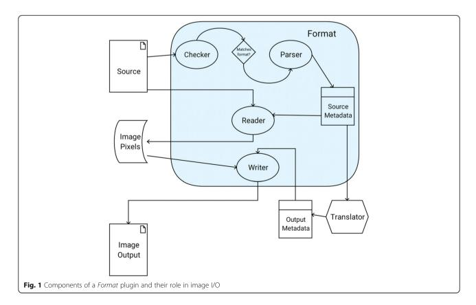
The *Checker* component contains the logic for matching a given *Format* with a potential image source, while the *Parser* component performs the actual creation of *Metadata* from that source. The *Reader* and *Writer* components use *Metadata* to read or write pixel data, respectively. Given the goal of freely shareable image data, *Writers* are optional components and should not be implemented for proprietary formats.
