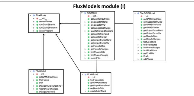
Fig. 3 FluxModels module class diagram (part I). The FluxModels module contains classes for the different types of models used for each flux analysis type: FBA, <sup>13</sup>C MFA, 2S-<sup>13</sup>C MFA, ELVA, etc. *Arrows* indicate derived classes
