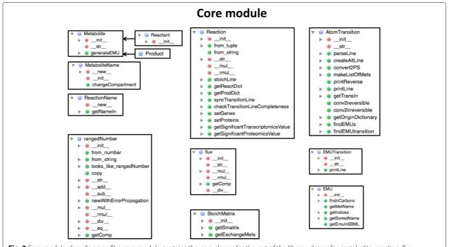
**Fig. 2** Core module class diagram. The core module contains the core classes for the rest of the library: classes for metabolite, reaction, flux, elementary metabolite units (EMU), atom transitions, emu transitions and stoichiometry matrices
