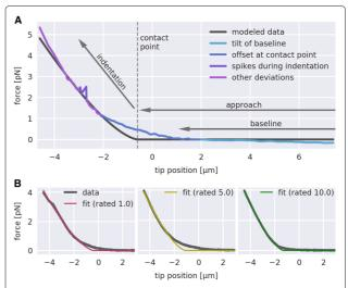
**Fig. 1** Rating of force-distance (FD) curves. **a** Visualization of several features that degrade the quality of FD curves. **b** Three FD curves with corresponding fits according to Eq. 3 are shown. The colors of the fit label the manual rating (1/magenta: poor, 5/yellow: acceptable, 10/green: good)
