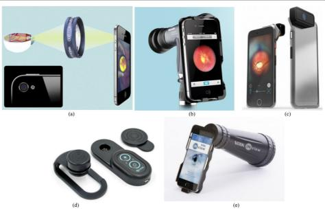
**Fig. 1** Smartphone-based retinal imaging systems available in the market, **a** Fundus photography method used by Harvard Medical School **b** iExaminer developed by Welch Allyn, **c** D-Eye, **d** Peek Retina, and **e** iNview by Volk
