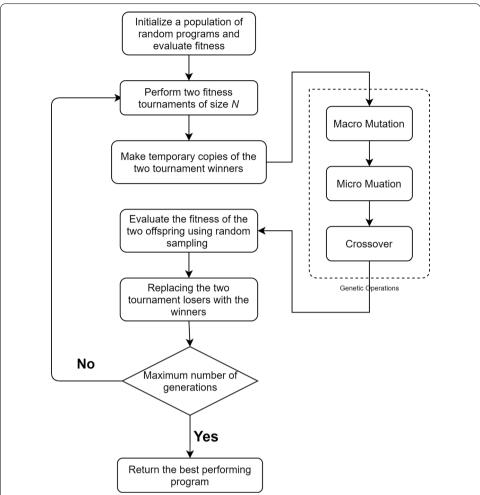
**Fig. 2** LGP algorithm flowchart. After initialization, this evolutionary algorithm repeats the processes of parent selection, mutation, crossover, and replacement, until the generation limit has been reached
