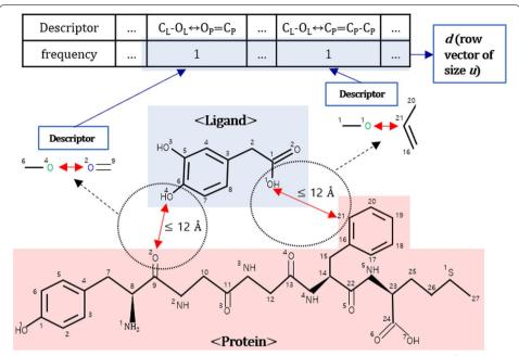
**Fig. 4** Example of descriptor. There are two atom pairs between which the distance less than 12 Å, and from which two descriptors can be identified. The frequencies in the protein–ligand complex are counted for all the unique descriptors in the training dataset, with the results being d. Note that OH is regarded as O, and atoms that are not specified are carbon C
