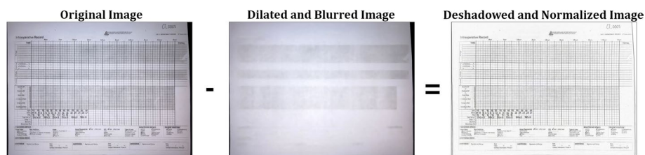
Fig. 2 Example of an anesthesia paper chart before and after the removal of shadows and normalization. The dilated, blurred image is subtracted pixel-wise from the original image to produce the final result
